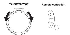
Adjusting the main volume adjusts the volume level of all the speakers connected to the TX-SR700/700E together. If headphones are connected, this also adjusts the volume heard from the headphone speakers. To adjust the volume, either press the VOL  $\Delta/\nabla$  buttons on the remote controller or turn the MASTER VOLUME dial. To increase the volume, turn the dial clockwise; to decrease the volume, turn the dial counterclockwise. The volume can be set to Min, 1 to 99, and Max.
